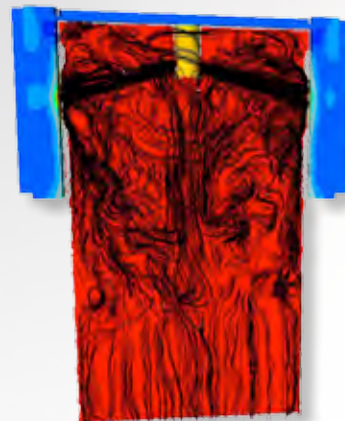
Illustrating liquid metal paths and checking mold temperatures using cooling channels during the process
