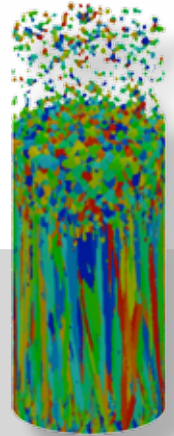
Grain structure in volume under driven solidification conditions
