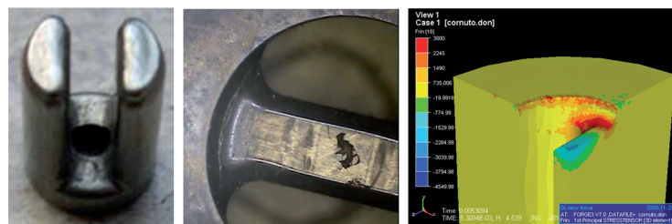
Fig. 10 – Analysis of the molds for the configuration of fork spanner cold forging (courtesy of Omega IFS S.r.l.)
