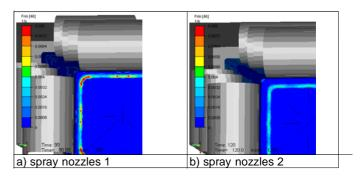
Fig. 4 : Yamanaka et al [3] criterion (cutting plane) for two different cooling patterns
