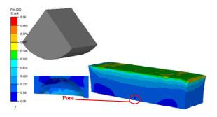
Fig. 7 : Forge2005® simulation of porosity evolution using an actual hole in the mesh (transient simulation)
