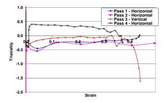
Fig. 8: Triaxiality rate versus strain evolution during rolling on the free surface
