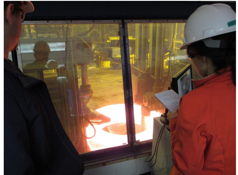
Radial-axial ring rolling at Scot Forge McHenry, Illinois
